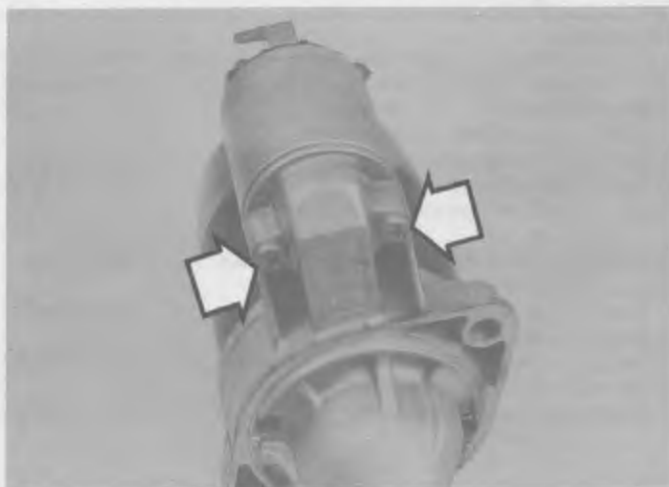
21.4 . . . then remove the solenoid mounting screws (arrows) and pull the solenoid straight off the starter flange
