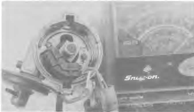
11.7 Measure the resistance of the igniter – if it isn't as specified, replace it (1990 and earlier models)
