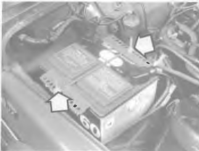
3.2 Unscrew the nuts (arrows), then pull the hold down clamp off the battery
