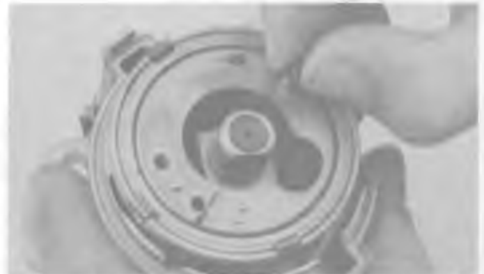
13.5c When lifting the generator base plate out of the distributor body, be careful not to nick the signal rotor teeth
