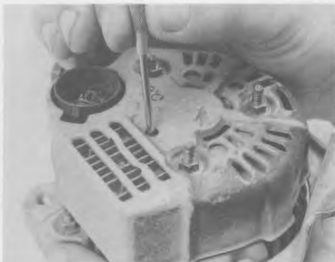
15.6 If the charging voltage is low, insert a metal tool into the test hole in the rear of the alternator and take a voltage reading at the B+ terminal on the alternator – if the voltage rises, the regulator is faulty (alternator removed for clarity)
