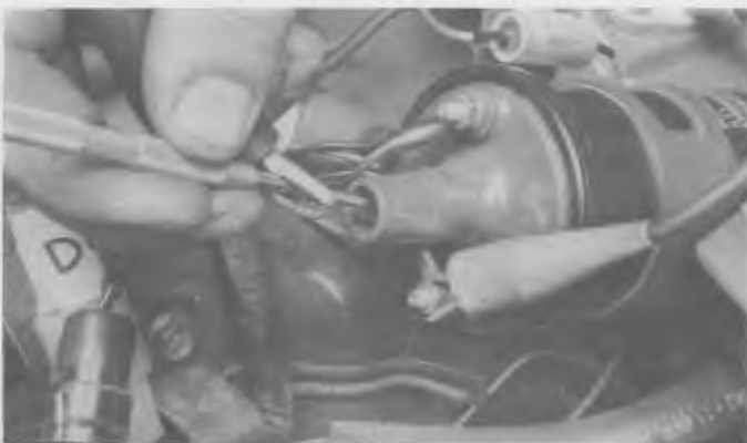
7.4 When measuring the secondary coil resistance, insert a probe into the coil tower and connect the other lead to the positive (+) primary terminal (1990 and earlier models)
