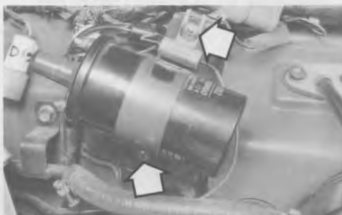
7.8 The coil is attached to the firewall with two screws (1990 and earlier models)
