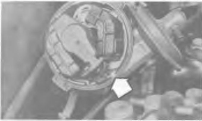
8.5a Before removing the distributor, use chalk or a felt-tip pen to make an alignment mark on the edge of the distributor base directly beneath the rotor tip – DO NOT use a lead pencil
