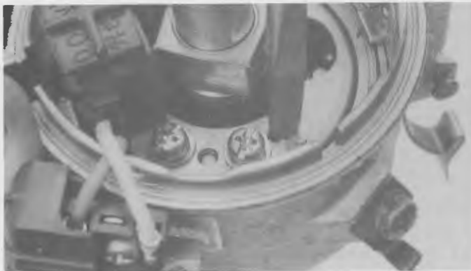
12.3 The air gap can be adjusted by loosening the two igniter screws, inserting a screwdriver into the slot in the igniter and turning the screwdriver to pry the igniter toward or away from the signal rotor
